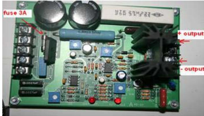
3- Check the signal at the output of the board using an oscilloscope. You will find a square wave with amplitude 170v. If not, replace the board (board burned).
