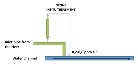
With the gates and the inlet flowrate we can control the contact time of ozone in the water. TEST N°2:
