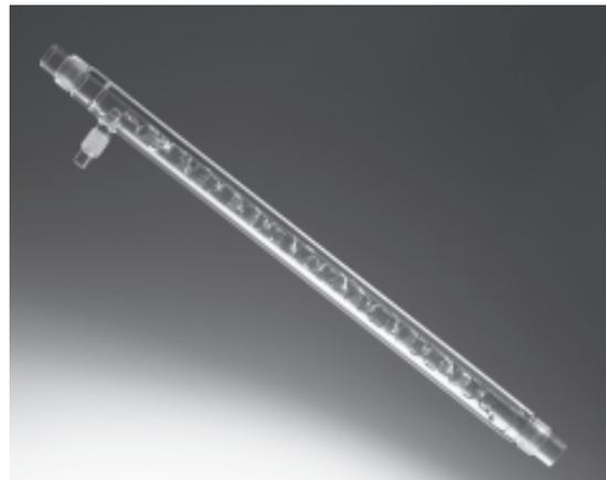
Figure 3. An example of a static mixer.
